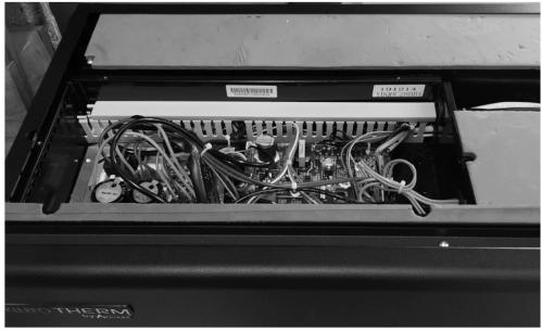
5. Locate the 2 fixing points and the 4-pins "blue" connector
