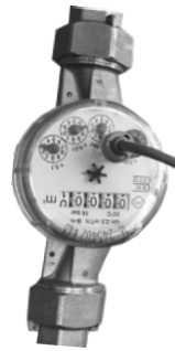
Figure 45. Connecting the water meter to flow input 1( red wire on terminal 1 and black wire on - )
