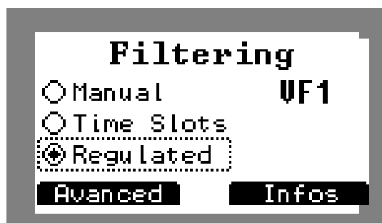
Figure 10. Regulated mode setting screen
