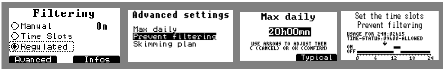
Figure 4. Filtering programming screens in regulated mode
